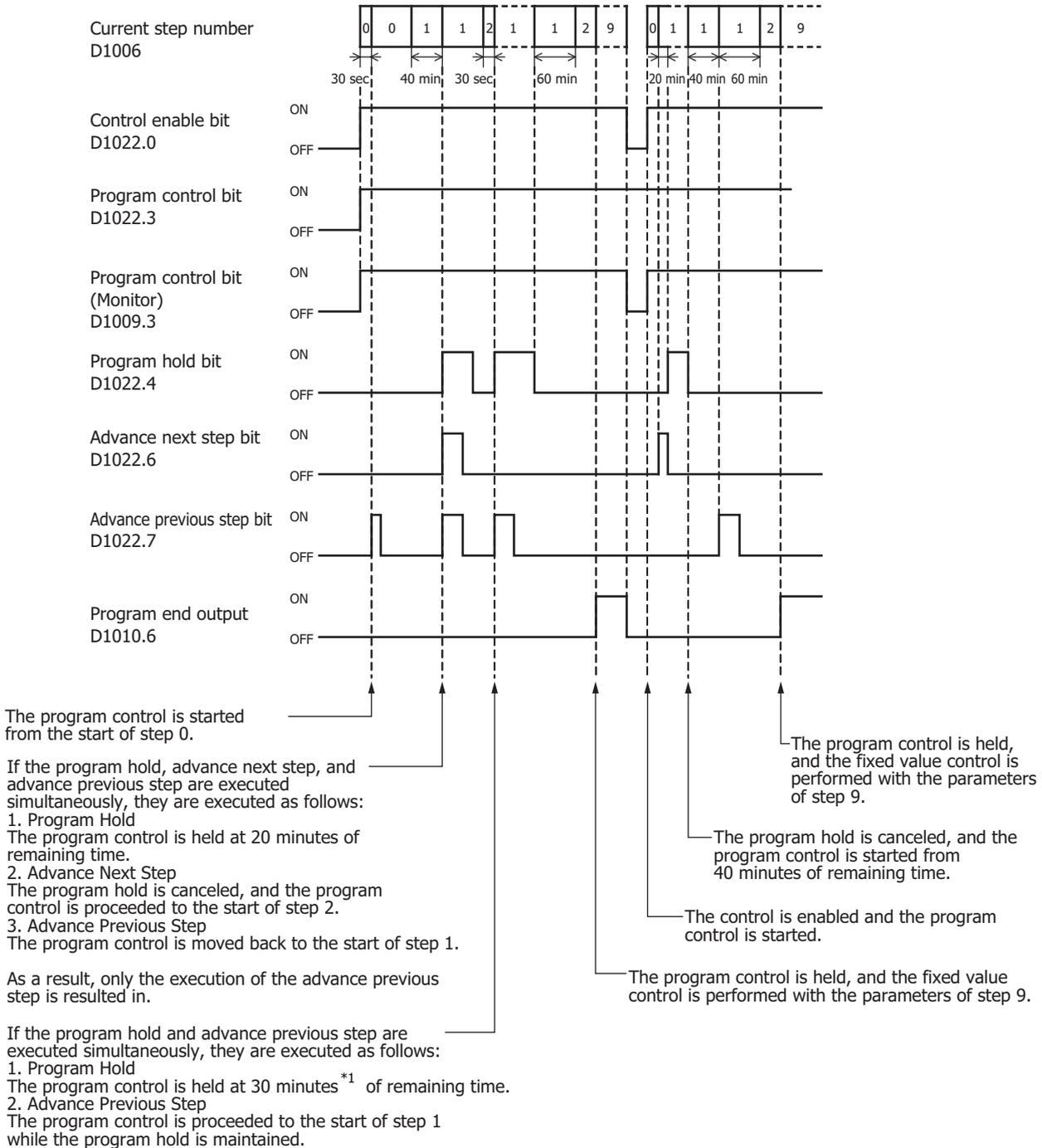
\*1 If minute is selected as the step time unit, the remaining time is handled with the unit of minute. If the remaining time is between 29 minutes 1 second and 30 minutes 0 second, the remaining time will be 30 minutes.
