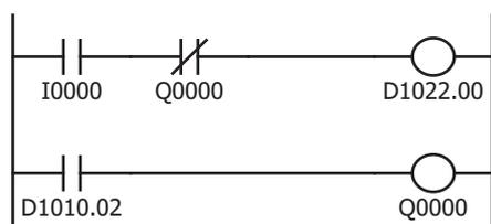
When external input I0 is turned on, CH0 control is enabled. When Q0 (loop break alarm output of CH0 control) is turned on, CH0 control is disabled.
