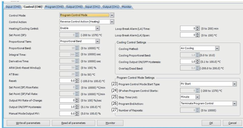
Control parameters of CH0 control are described here. When the program control mode is selected as the control mode, parameters for the fixed value control mode, such as the set point (SP), proportional band/proportional gain, or integral time, are disabled. The parameters for the program control mode (23) to (27) are enabled.
