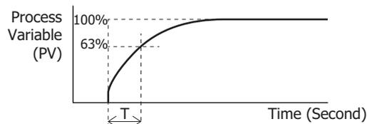
Figure 2. Process variable (PV) after PV filtering process
