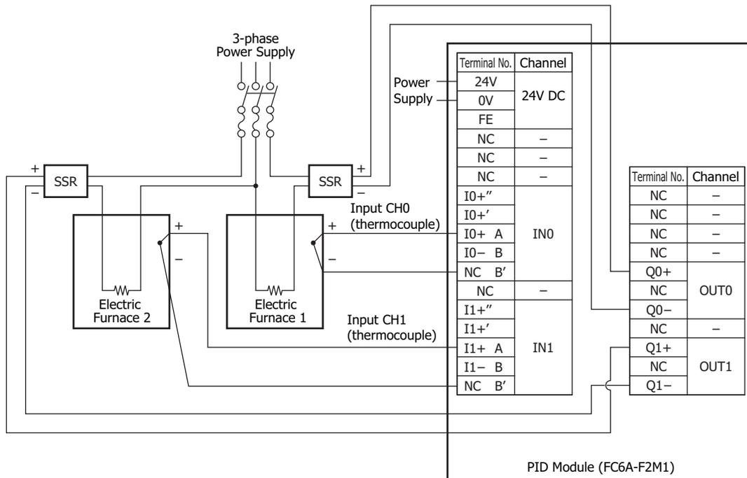
**PID Module Parameter Configuration**
