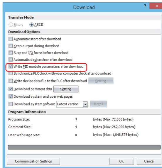
When the **Write PID module parameters after download** check box is selected, after the user program is downloaded to the CPU module, the parameters configured in the **PID Module Configuration** dialog box will be written to the data registers in the CPU module and the PID modules with the slot numbers that were inserted with the Module Configuration Editor.
