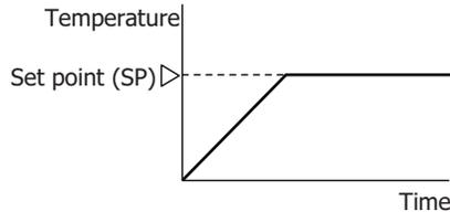
The program control allows you to define the set point (SP) that changes as the time progresses so that the process variable (PV) can be controlled to match the set point (SP) changing as the time progresses. The set point (SP) and time can be configured for each step. A maximum of 10 steps can be configured and performed. The set point (SP) can be configured as shown in the following diagram.
