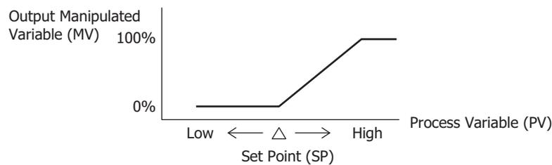
In reverse control action, the output manipulated variable (MV) increases when the process variable (PV) is lower than the set point (SP) (negative deviation). For example, electric furnaces perform the reverse control (heating) action.
