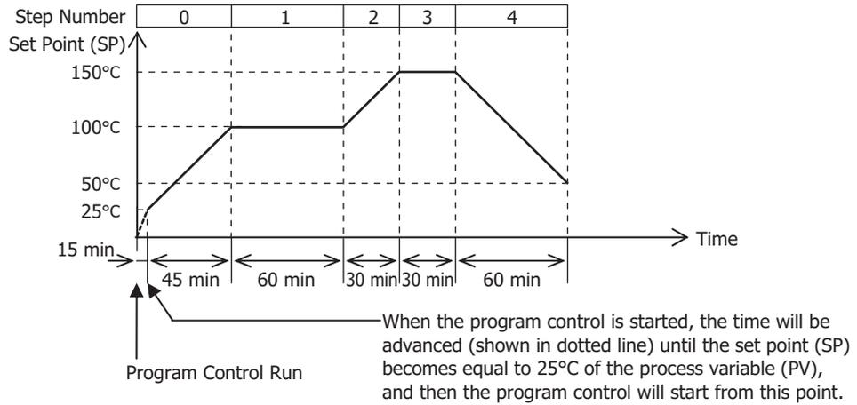
**PV Start Action [Process variable (PV) is 170°C]**
