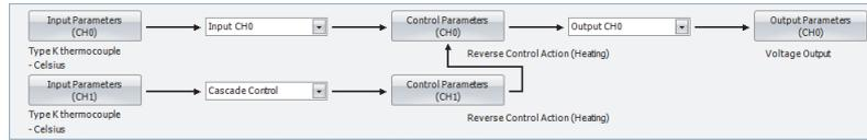
Master (CH1 control) calculates the output manipulated variable (MV) according to the process variable (PV) and the set point (SP). The output manipulated variable (MV) of the master (CH1 control) is used as the set point (SP) of the slave (CH0 control). With the obtained set point (SP), the slave (CH0 control) calculates the output manipulated variable (MV) and controls the output CH0.
