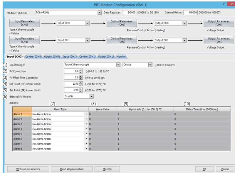
Input parameters for CH0 control are described here. Input parameters for CH1 control are the same as those of CH0 control. However, the position from the control register for each parameter differs. For details about the positions from the control register for CH1 control, see "Blocks 2, 3: Basic Parameters (SHOT Action)" on page 5-18 and "Blocks 4, 5: Initial Setting Parameters (SHOT Action)" on page 5-20.
