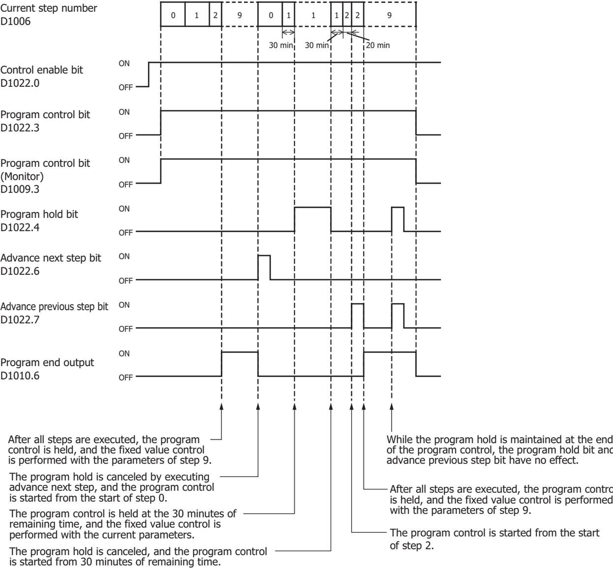
**Note:** The PID module executes all steps 0 to 9 even if the step times of steps are zero. When the program control is terminated, nine is stored in the current step number of Block 0.
