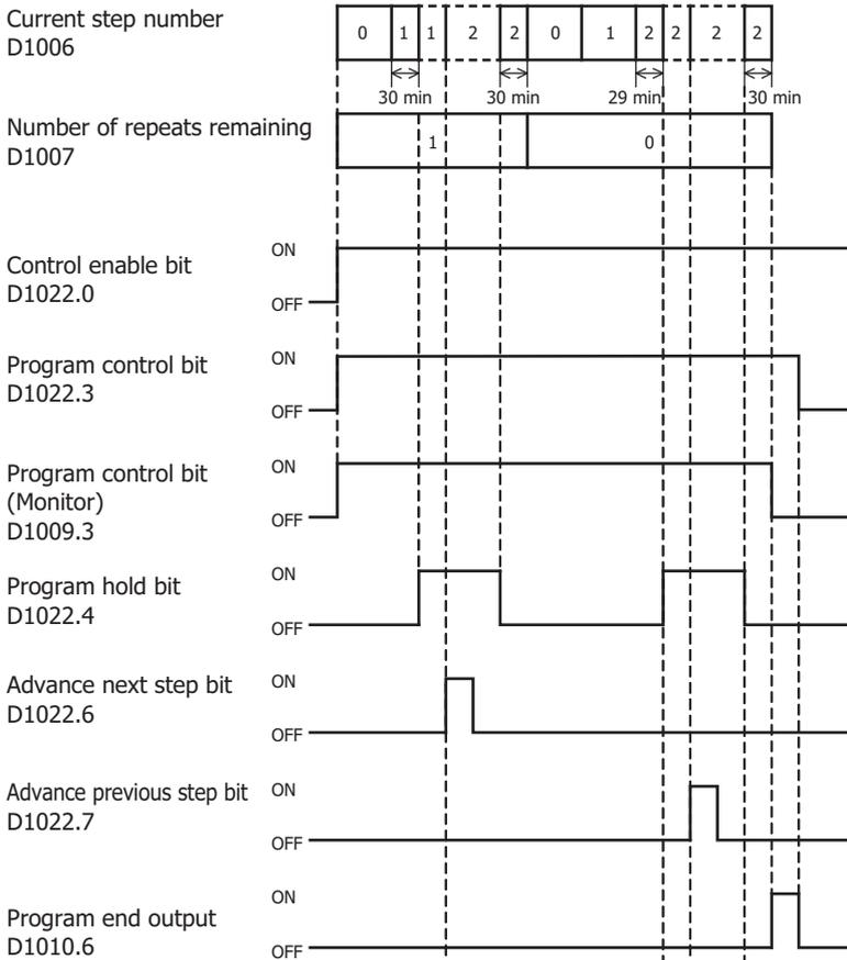
The program control is proceeded to the start of step 2 while the program hold is maintained.
