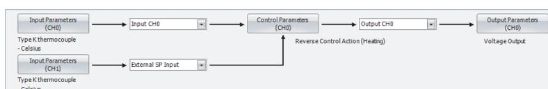
When the external SP input bias is configured, the external SP input bias is added to the input CH1 value, and then the input CH1 value is used as the set point (SP) for CH0 control. One of the analog input types shown in the table below can be selected for the external SP input.
