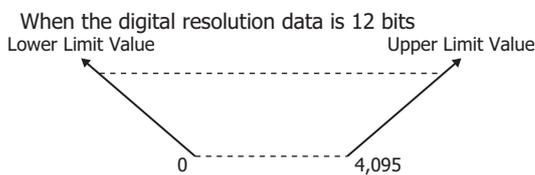
\*2 Input data out of range is reflected in the status of the analog I/O module.
