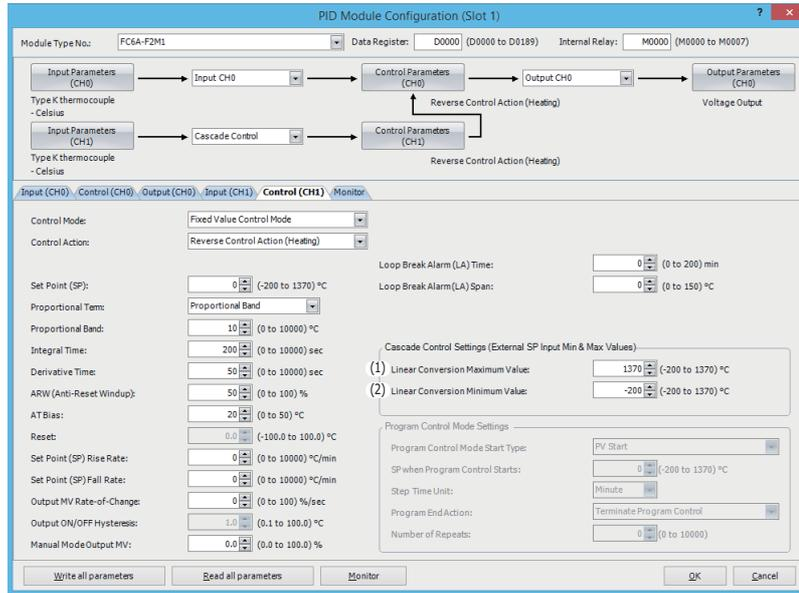
**(1) Control Register+178: External SP Input Linear Conversion Maximum Value**
