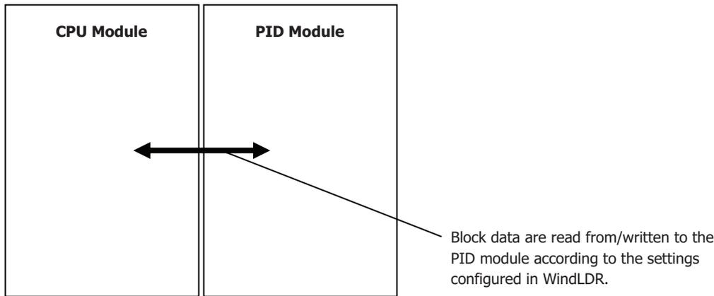
The PID module parameters consist of 26 data blocks divided according to the function and frequency of use of each parameter as shown in the table below. All blocks to be used are allocated to the data registers in the CPU module. The parameters of each block can be read from/written to the PID module using the allocated control relays.
