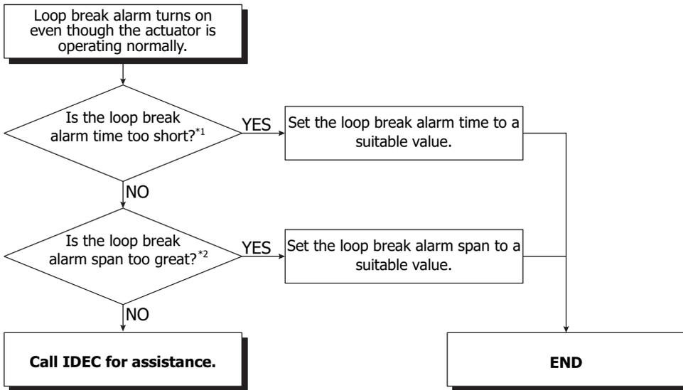
\*1 Loop break alarm time may be too short compared to the loop break alarm span.
