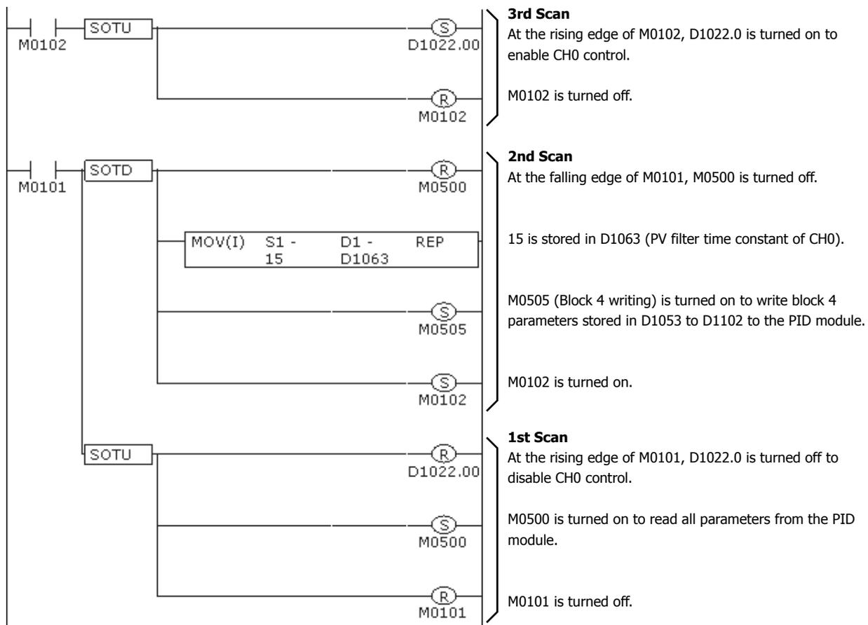
\*1 If the reading all parameters (M0500) is turned on, all PID module parameters are read out from the PID module and stored in the data registers. Block 4 parameters are stored in D1053 to D1102.
