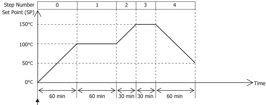
When the program control is started, the program control will start from 0°C of the set point (SP) configured with "Set Point (SP) when Program Control Starts" regardless of the current process variable (PV).
