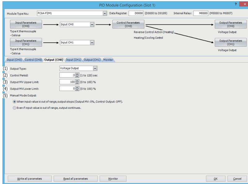
Output Parameters when Heating/Cooling Control is Enabled
